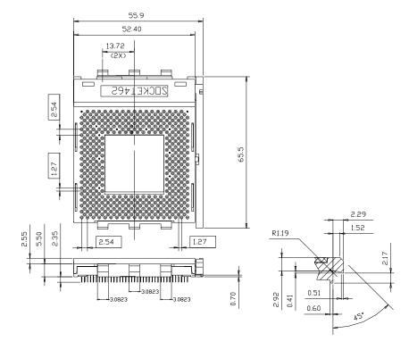
Figure 2. Dimensions of Socket A
