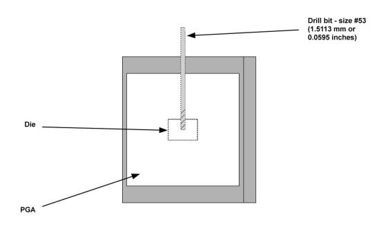
Figure 8. Bottom View of Heatsink and Drill Depth
