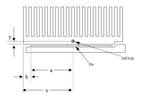
Figure 7. Measuring Thermocouple Position
